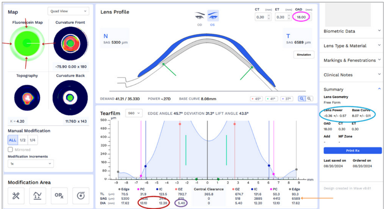
Fig. 5: Second lens design. The sagittal height in the temporal area of 6589 \mu\text{m} (orange arrow). The green and red arrows indicate the scleral lens vaulting the limbus. In the lens profile on the ocular surface, the scleral lens is now vaulting the limbus (green arrows). On the fluorescein map, no black areas are seen anymore (red arrows). To clear the limbus, the chamber diameter was increased by moving the blue (IC) and pink (PC) dots (red circle) outward. Lens power was reduced to -0.36 D by flattening the base curve to 8.07 mm (blue circle). To reduce corneal peripheral clearance, the optic zone diameter was reduced to 5.40 mm (purple circle).
